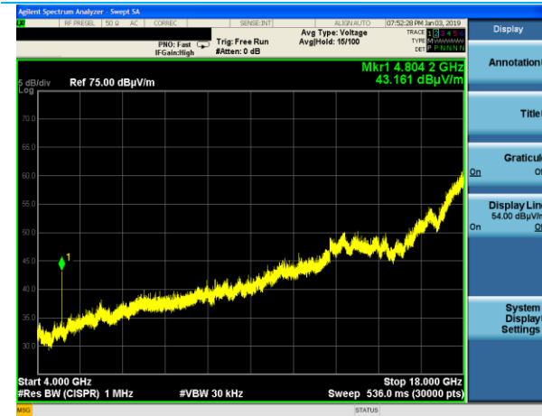
4-18 GHz, Horizontal Antenna, Vertical EUT, BLE Low Channel, Reduced VBW
