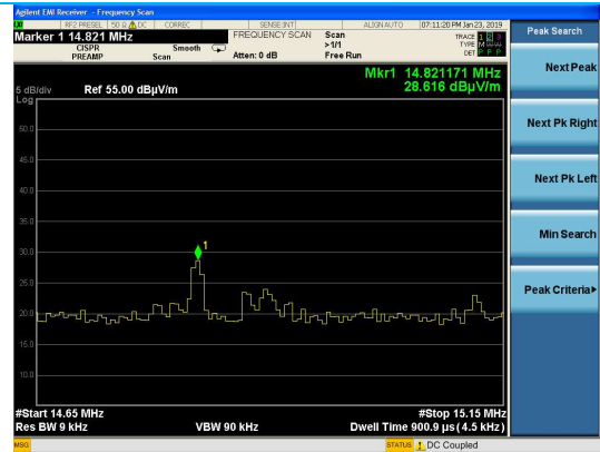
14.8 MHz Fundamental, Flat EUT Orientation Parallel Antenna Polarization
