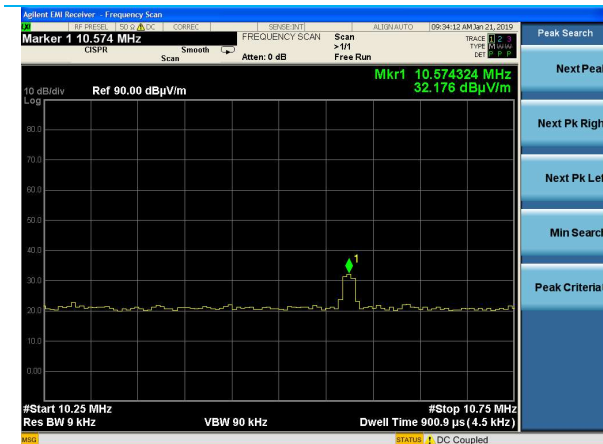
10.5 MHz Fundamental, Vertical EUT Orientation Perpendicular Antenna Polarization
