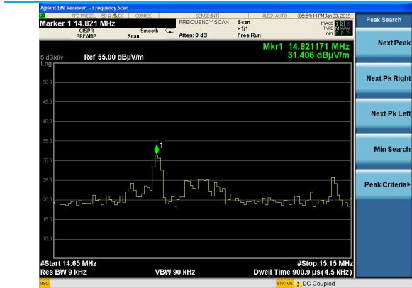
14.8 MHz Fundamental, Vertical EUT Orientation Perpendicular Antenna Polarization
