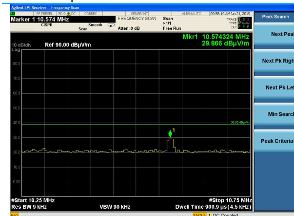
10.5 MHz Fundamental, Flat EUT Orientation Flat Antenna Polarization
