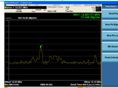
NFMI 14.8 MHz, Units Together Output Power
