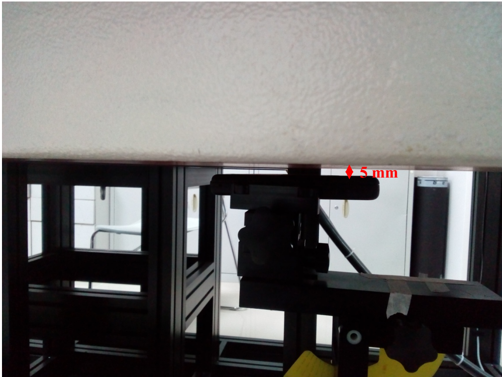
Body (Worn) Back Setup Photo (5mm)
