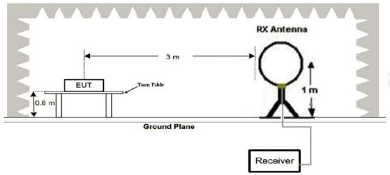
2. Radiated Emission Test-Up Frequency 30MHz~1GHz
