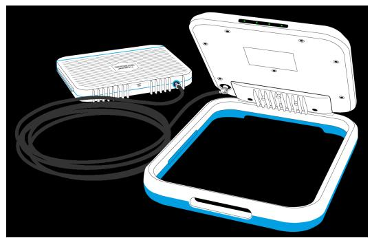
3. To change the cable on Thuraya SatBridge, put the cable removal tool under the cable connector and pull the tool up until the end comes out from SatBridge terminal. Do the same step on the other end of the cable. Now, bring new cable to be replaced, press each end of the cable connectors on the unit, as shown above and the connector should click into place.
