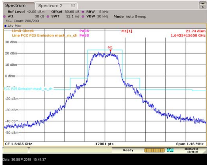
Figure 8.3-5: Emissions Mask M channel (QPSK)
