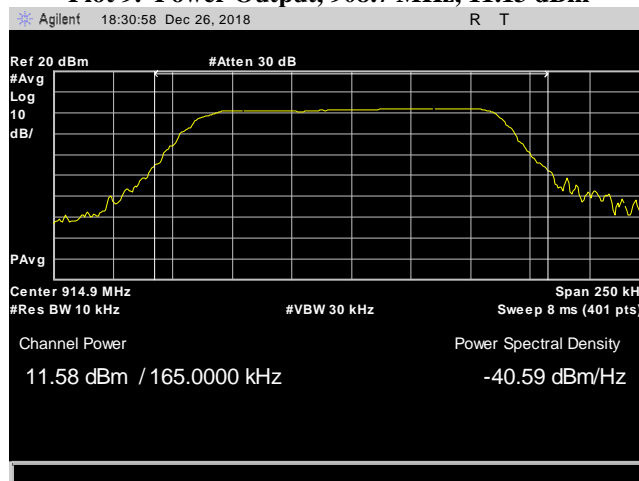
Plot 10. Power Output, 914.9 MHz, 11.58 dBm
