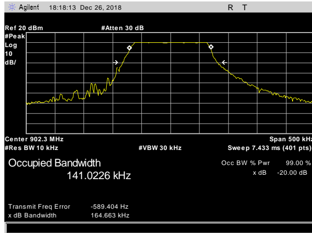
Plot 1. 20 dB Occupied Bandwidth, 902.3 MHz, 164.663 kHz
