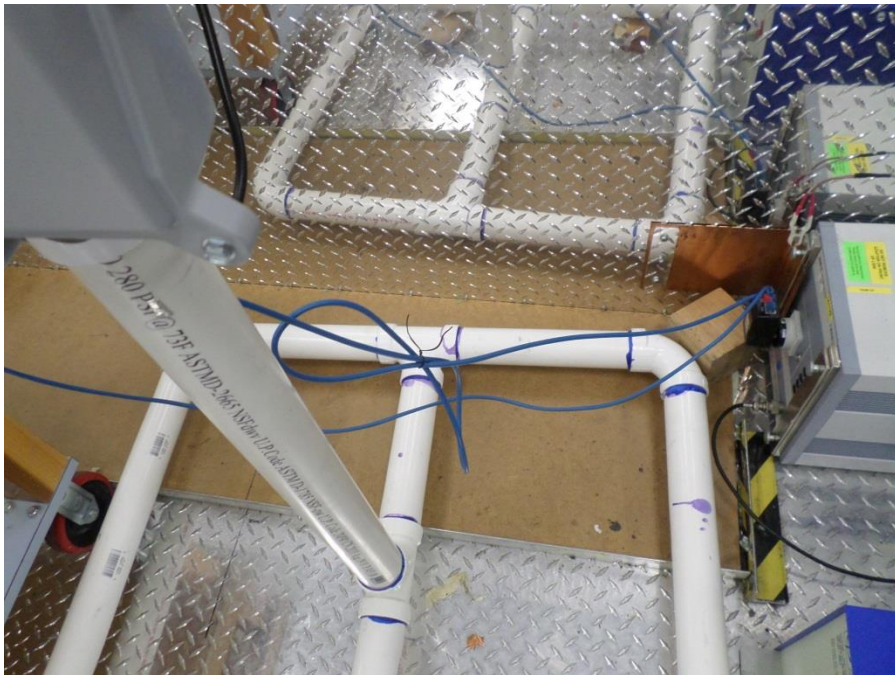
Photograph 2. Conducted Emissions, LISN Connection
