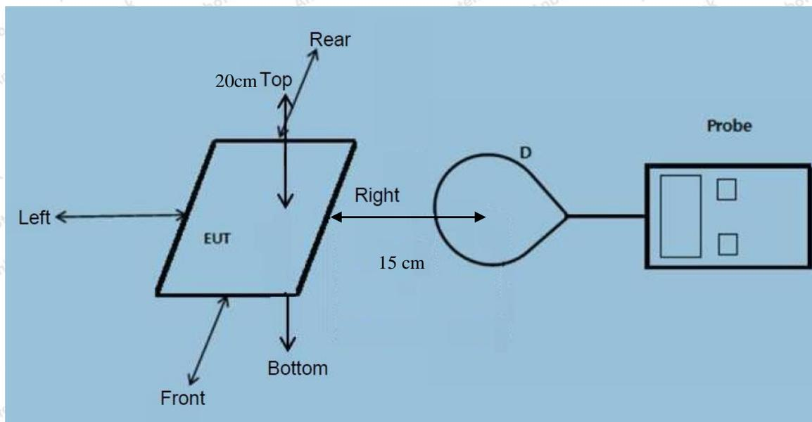
Note: Measurements should be made at 15 cm surrounding the EUT and 20cm above the top surface of the EUT.
