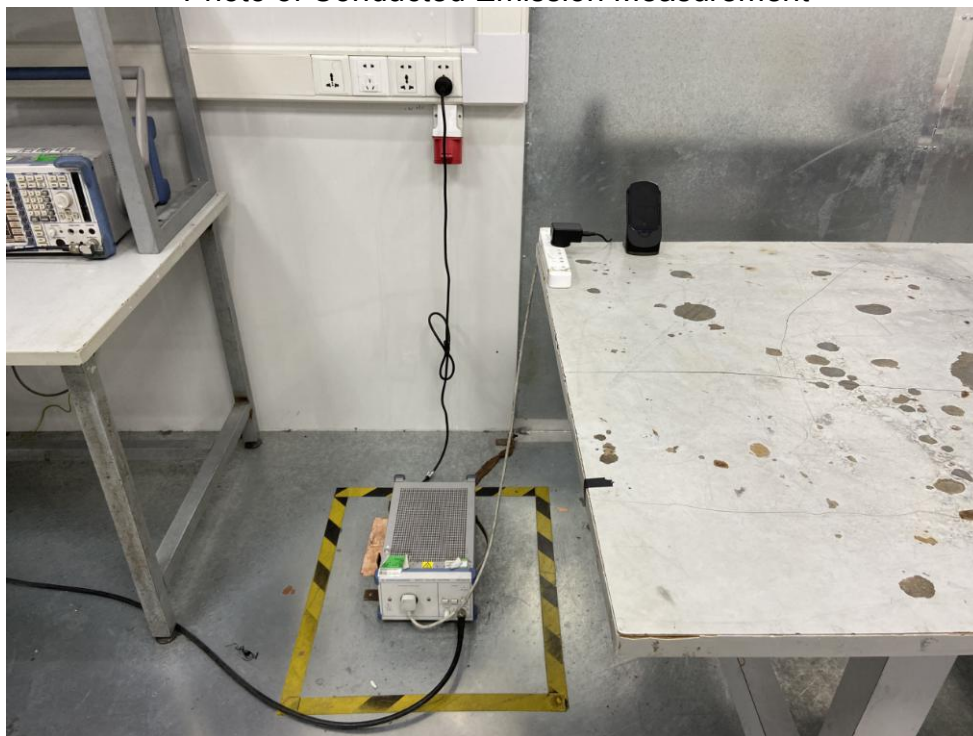
FCC ID: 2ARI5-MJ2-01 Photo of Conducted Emission Measurement
