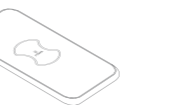
*Stick it on the back of the phone properly on the correct position with the help of the alignment film.
