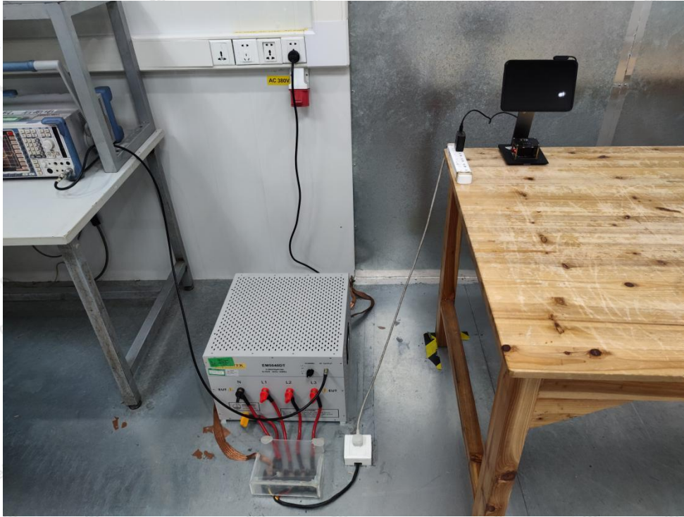
Photo of Conducted Emission Measurement
