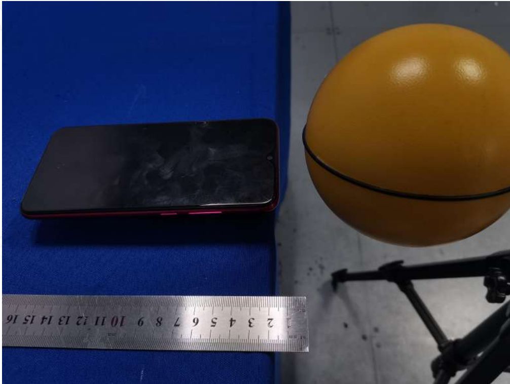
Test Position D(2cm) - Exposure photo from side edge surface-Front(TM1)
