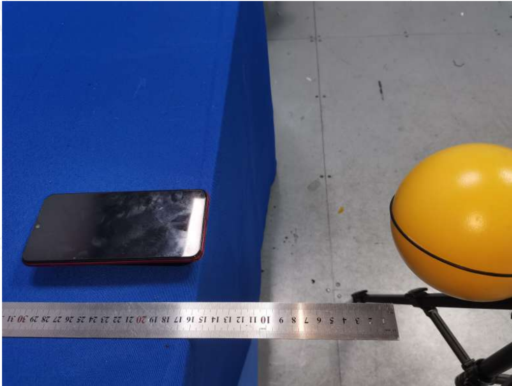
Test Position D(16cm) - Exposure photo from side edge surface-Front(TM1)
