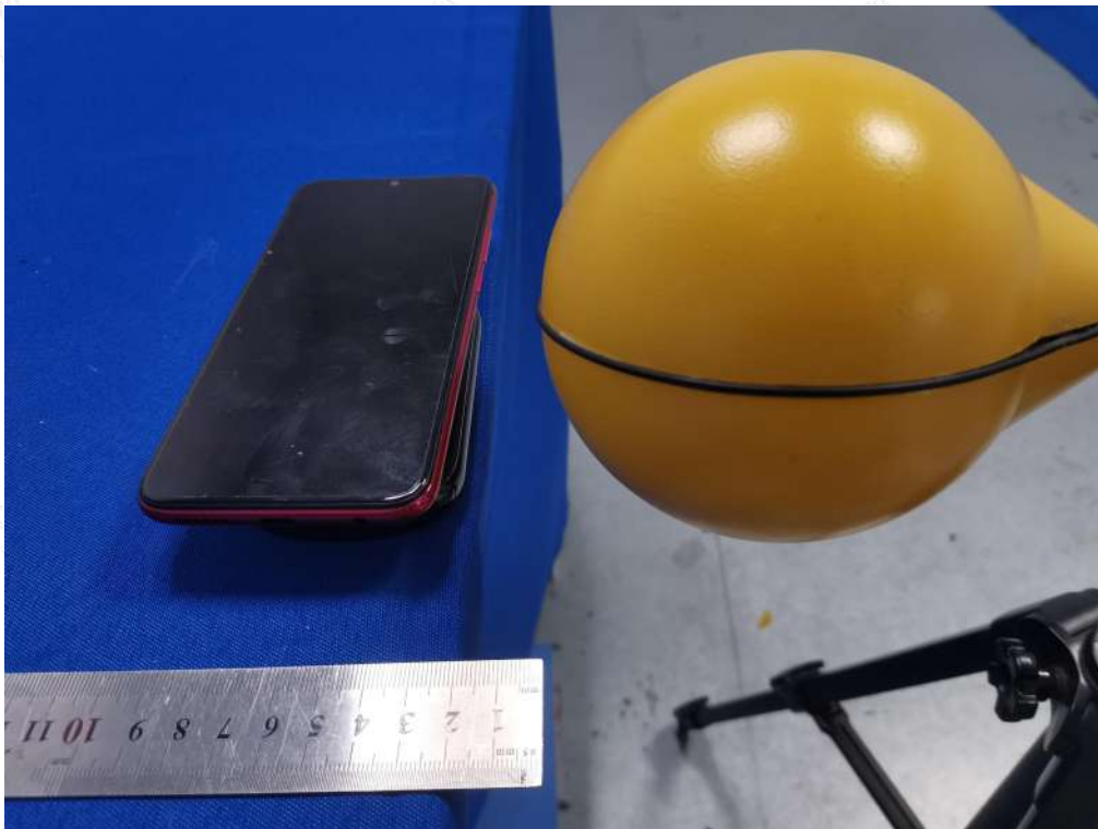
Test Position E(2cm) - Exposure photo from side edge surface-Right(TM1)
