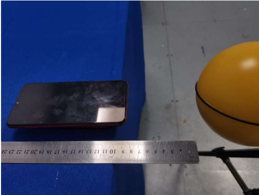
Test Position B(10cm) - Exposure photo from side edge surface-Rear(TM1)
