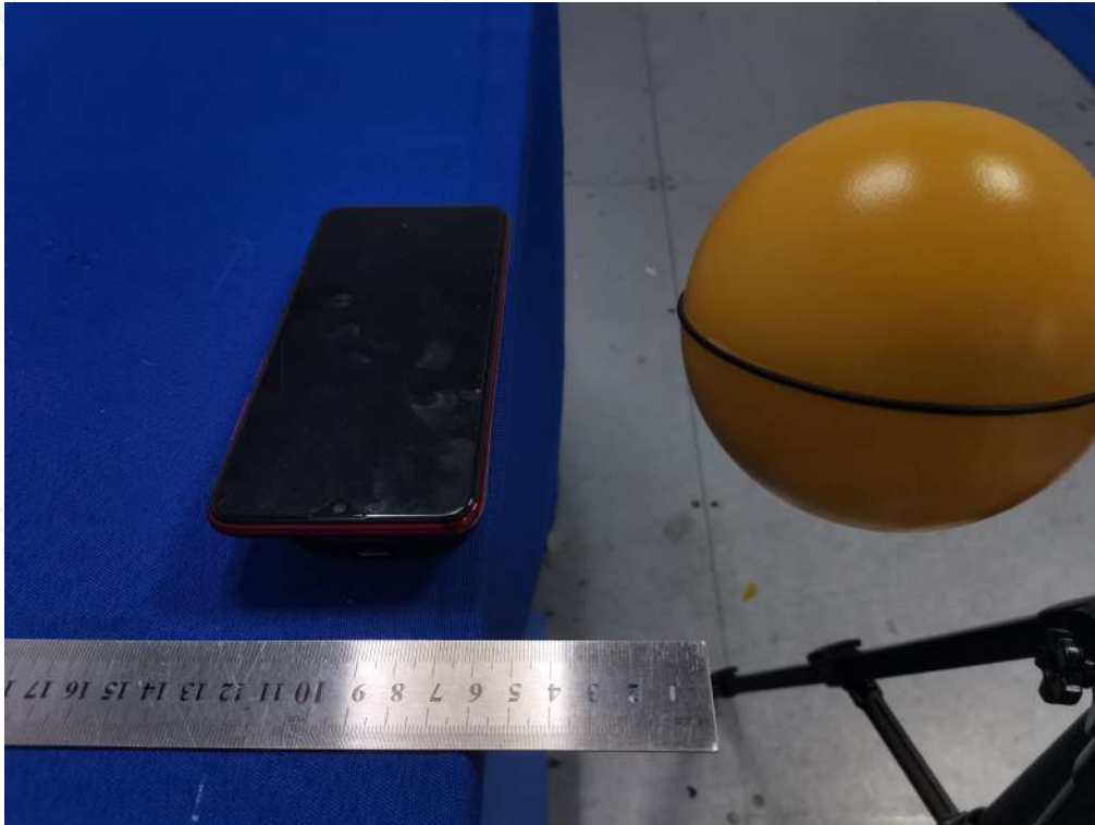
Test Position D(6cm) - Exposure photo from side edge surface-Front(TM1)
