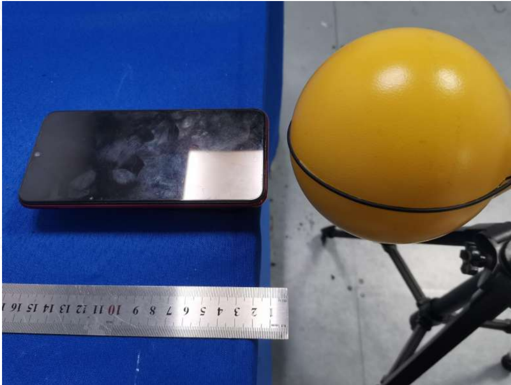
Test Position B(2cm) - Exposure photo from side edge surface-Rear(TM1)
