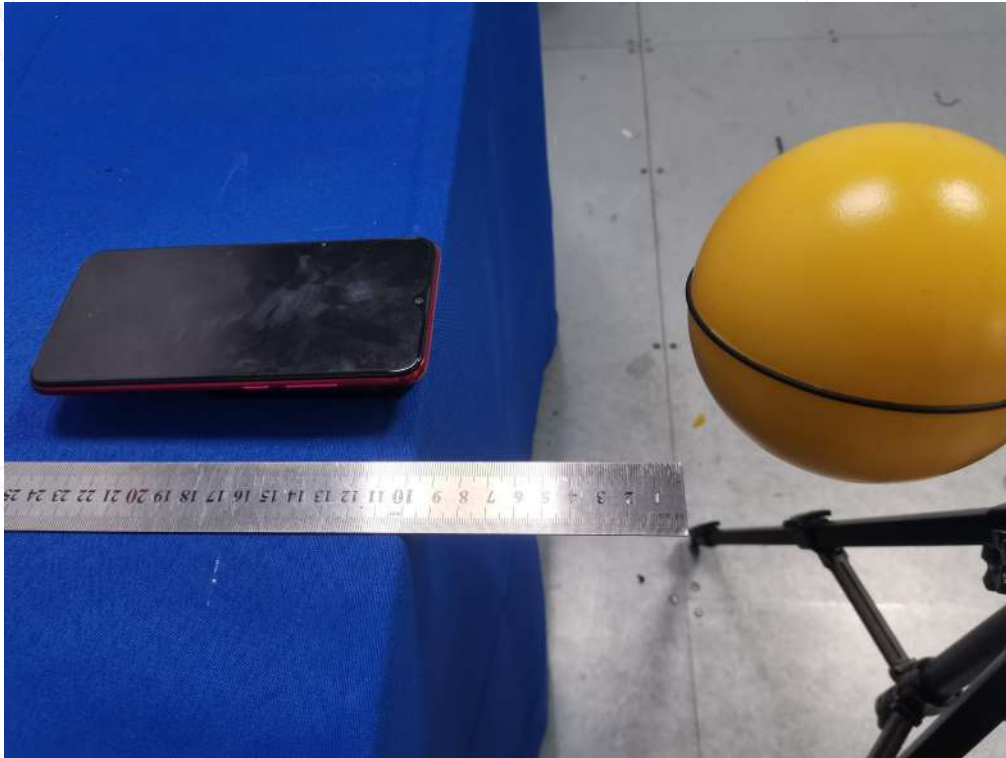
Test Position D(10cm) - Exposure photo from side edge surface-Front(TM1)
