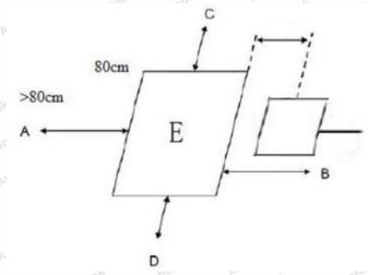
Note: Measurements should be made at 15 cm surrounding the EUT and 20cm above the top surface of the EUT. (probe radius is 4.75cm)
