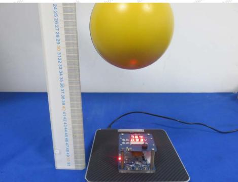
Photo of MPE Measurement (Conventional wireless charging)
