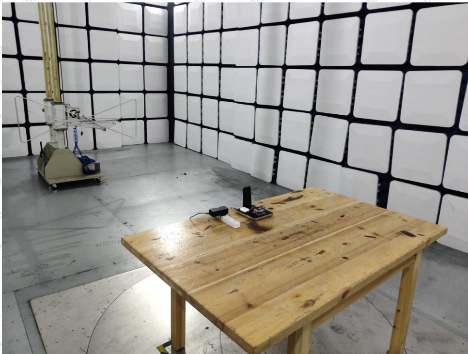
Photo of Radiation Emission Test
