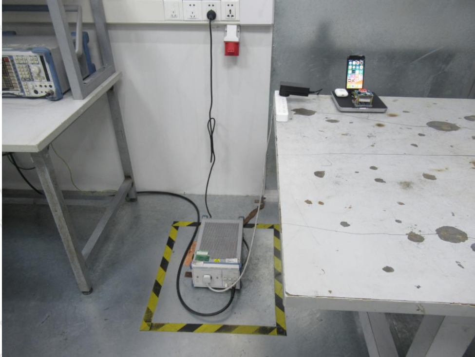
Photo of Conducted Emission Measurement
