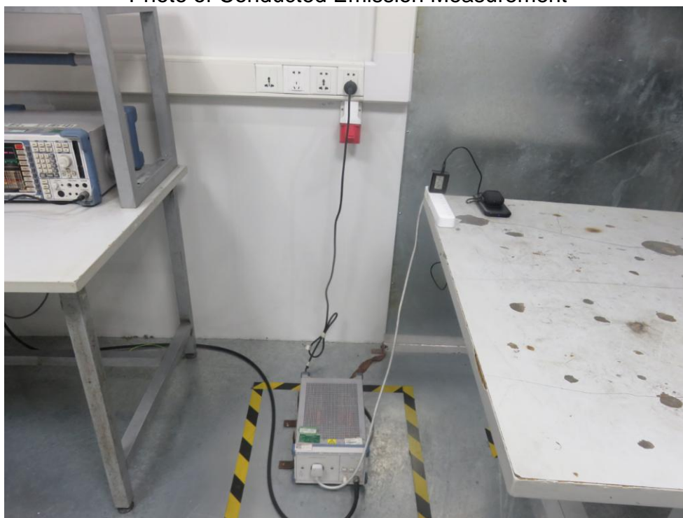
FCC ID: 2ARI5-APM1001 Photo of Conducted Emission Measurement
