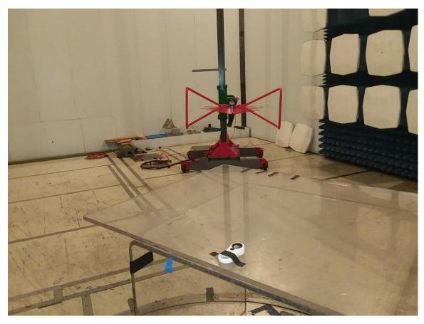
Photograph 2. Radiated Spurious Emissions, 30-1000 MHz, Test Setup
