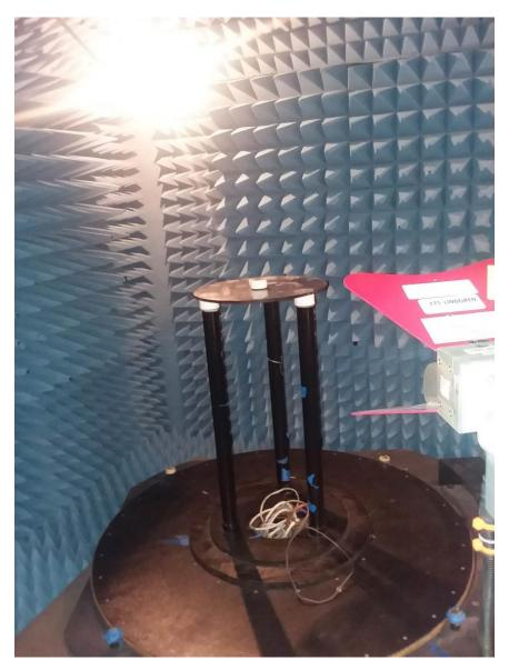
Photograph 1. Radiated Spurious Emissions, 1-18 GHz, Test Setup
