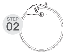
Keep pressing the AUTO icon and bumper for 3 seconds until a sound comes out
