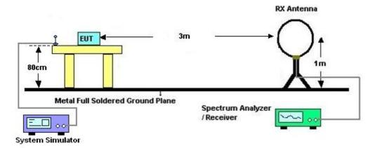
For radiated test from 30MHz to 1GHz
