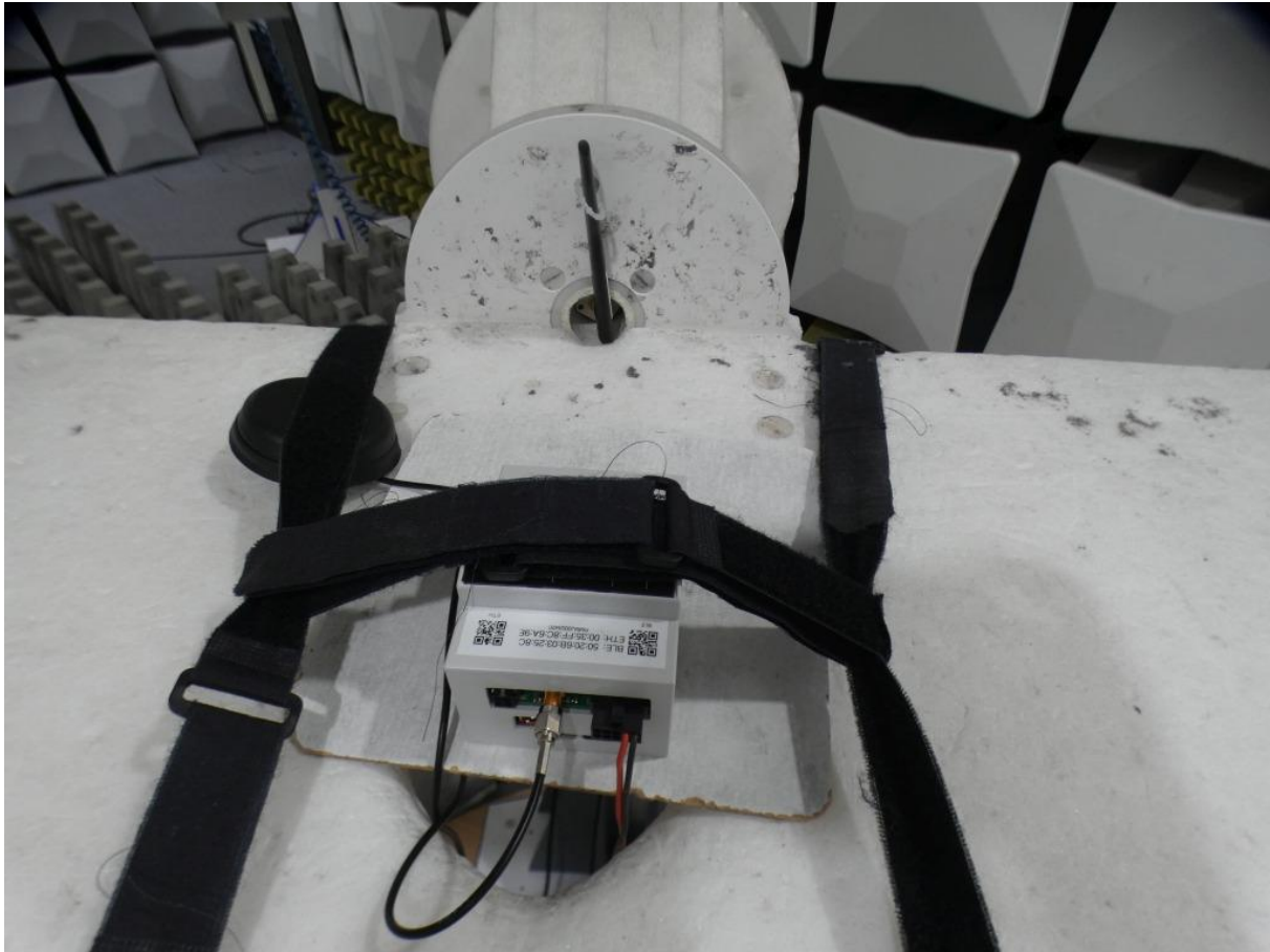
Photo 7: Test setup for radiated measurements, detailed view (stand alone setup, 1 GHz – 24 GHz; FCC 15c247)
