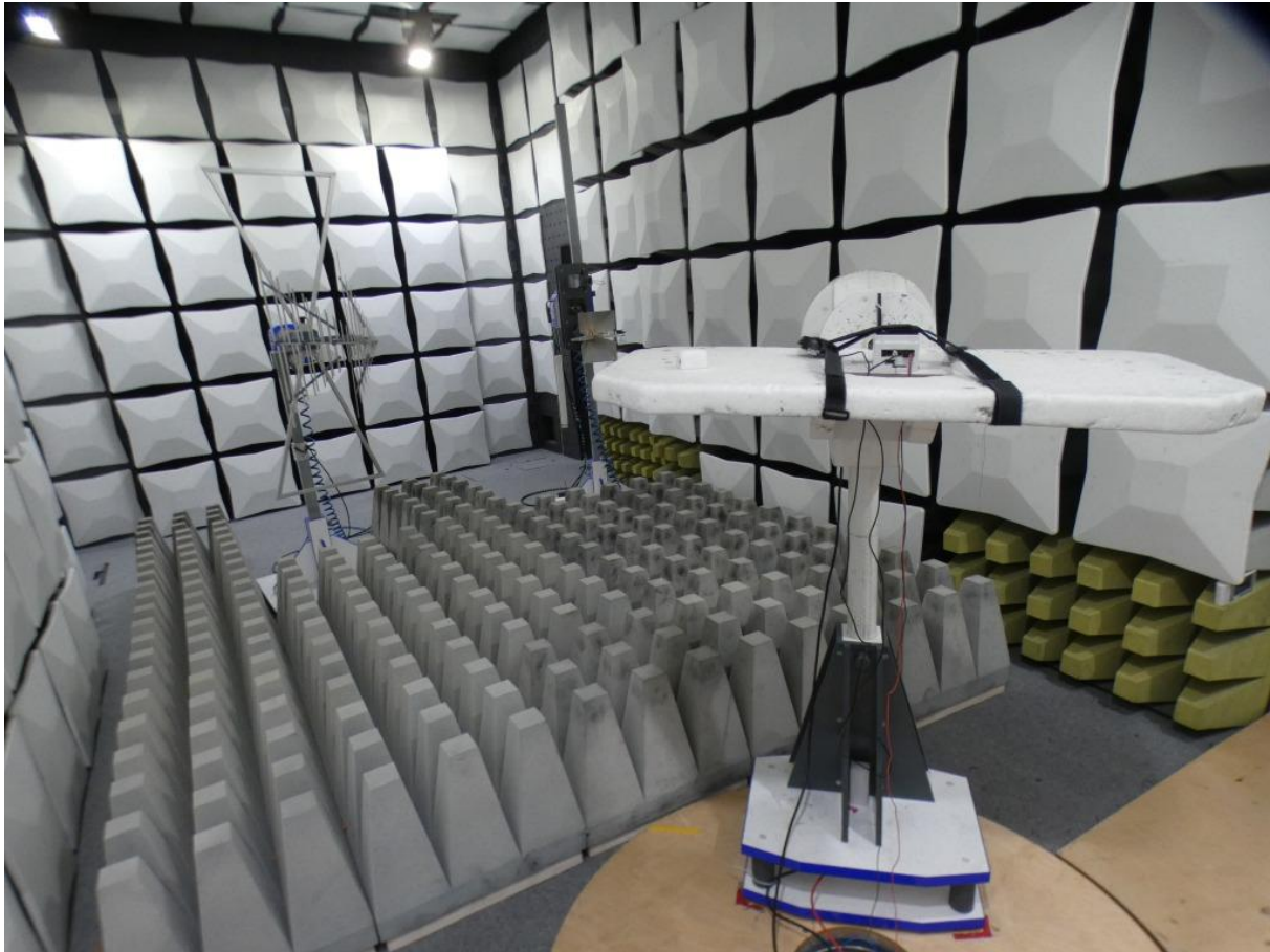
Photo 6: Test setup for radiated measurements (stand alone setup, 1 GHz – 24 GHz; FCC 15c247)
