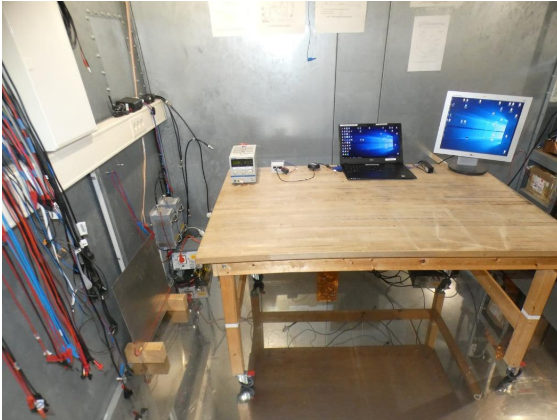
Photo 1: Test setup for conducted emissions (Computer peripheral setup, 150 kHz – 30 MHz; unintentional radiator §15.107, ANSI C63.4)
