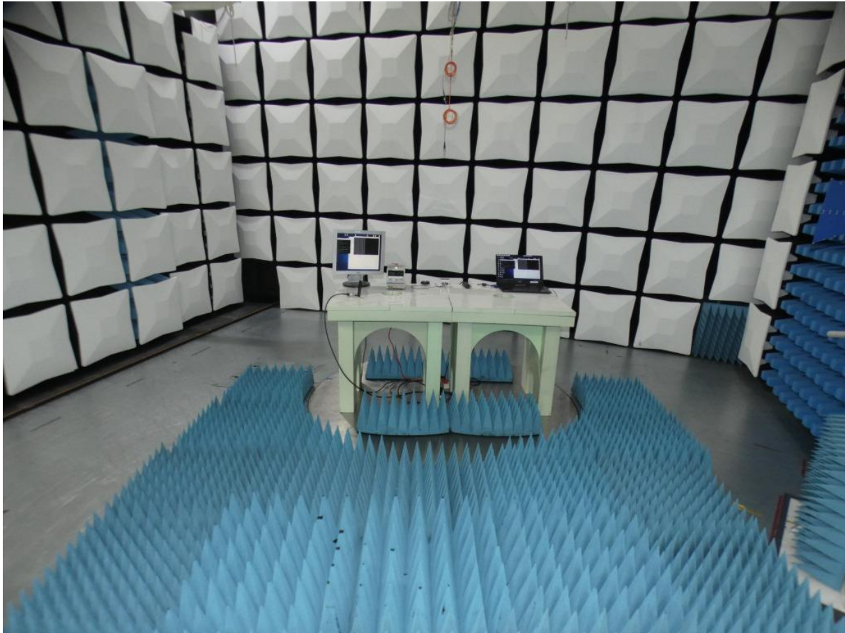
Photo 3: Test setup for radiated measurements (Computer peripheral setup, semi-anechoic chamber above 1 GHz ; unintentional radiator §15.109, ANSI C63.4)
