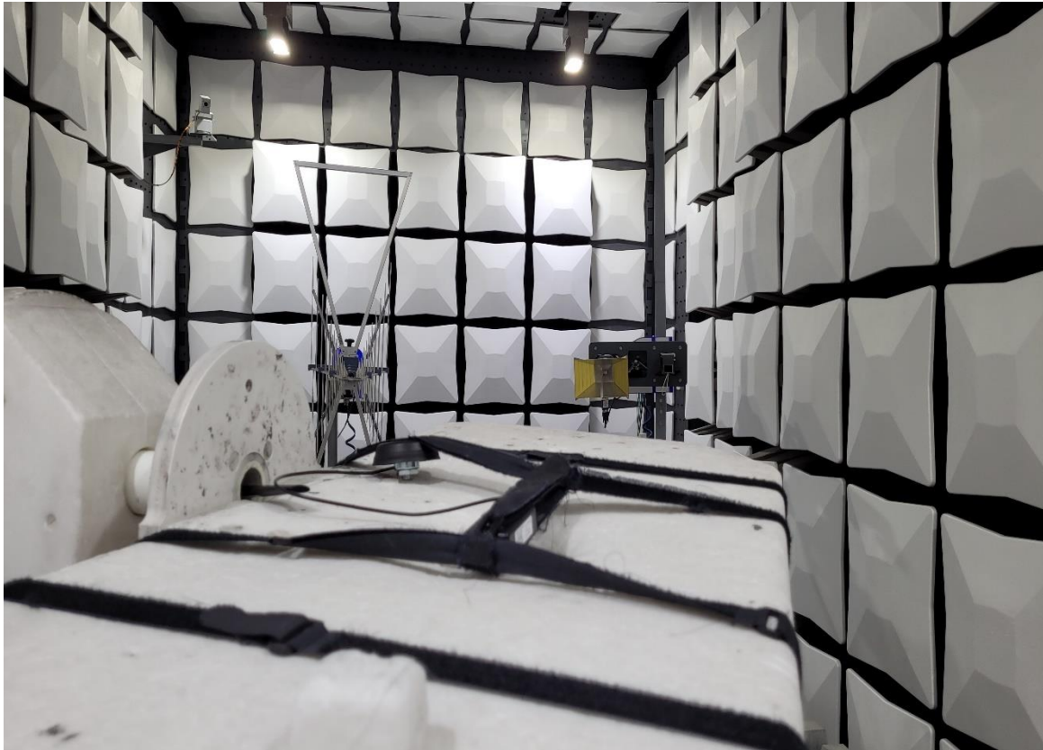
Test setup from EUT with 2J6602B antenna, detailed view (stand alone setup, 1 GHz – 24 GHz; FCC 15c247)
