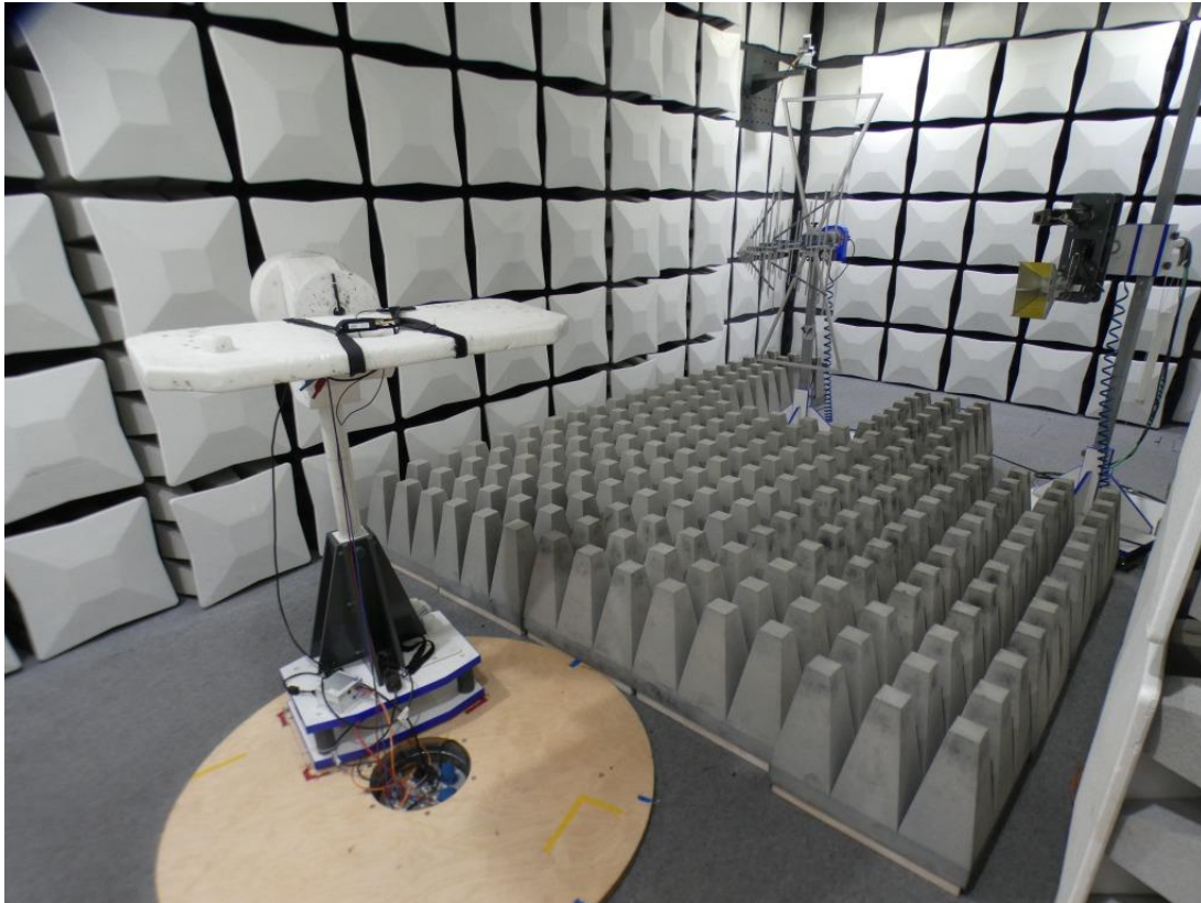
Photo 5: Test setup for radiated measurements (stand alone setup, 1 GHz – 24 GHz; FCC 15c247)
