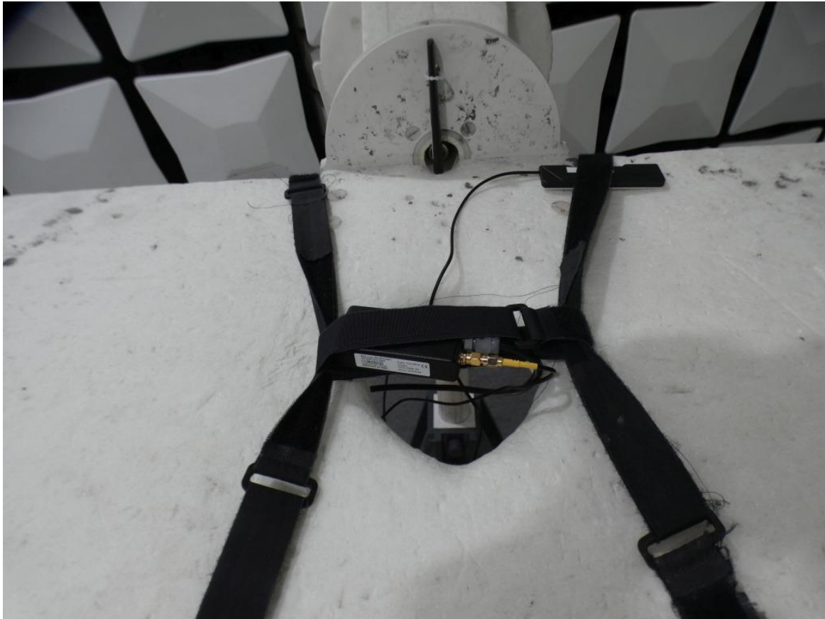
Photo 6: Test setup from EUT with Taoglas antenna, detailed view (stand alone setup, 1 GHz – 24 GHz; FCC 15c247)
