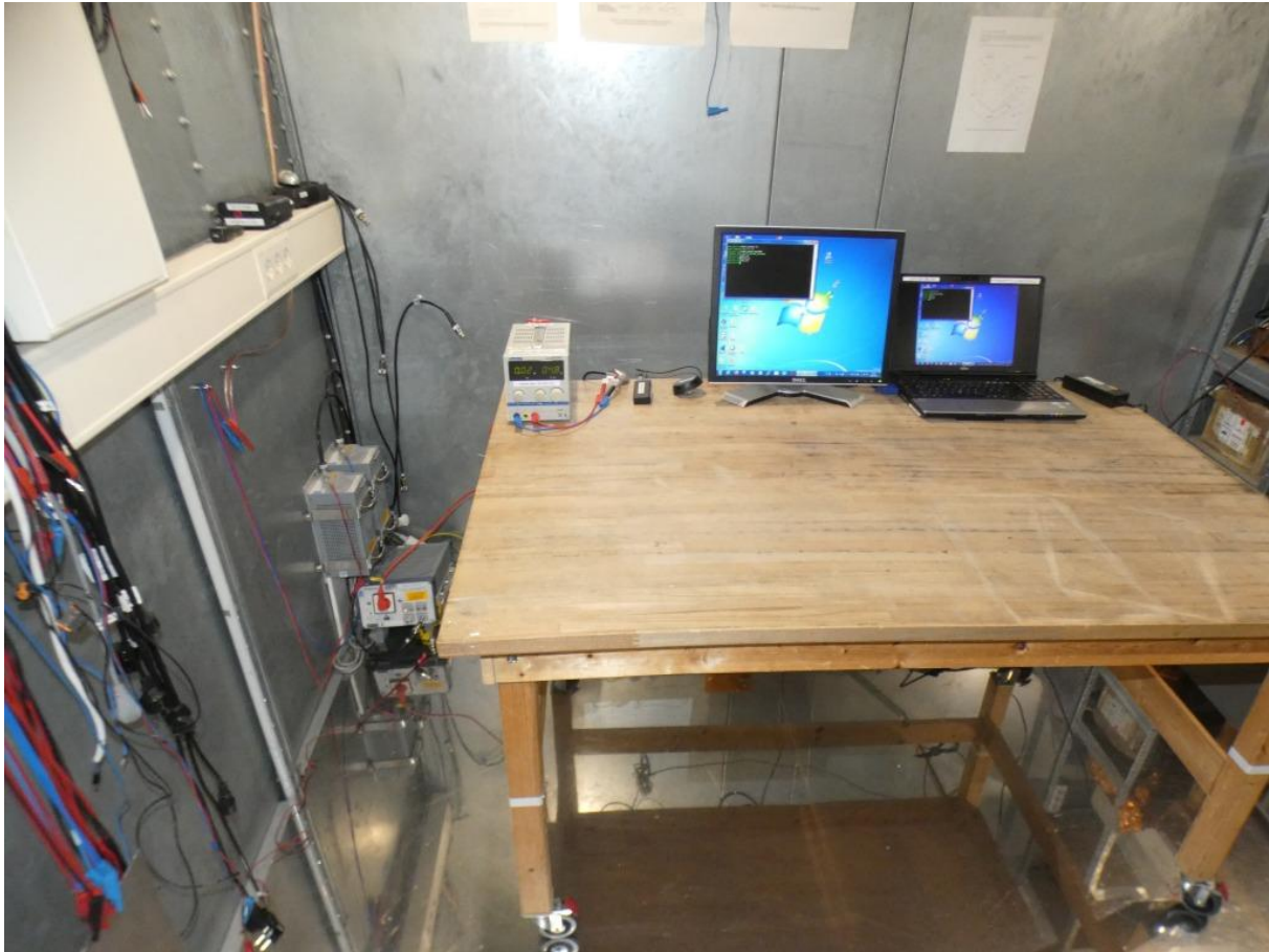
Photo 3: Test setup for conducted measurements (Computer peripheral setup, 150kHz – 30MHz ; unintentional radiato §15.107, ANSI C63.4)
