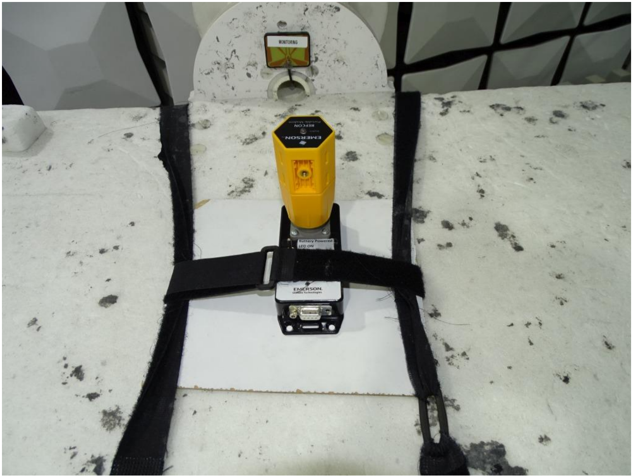
Photo 5: Test setup for radiated measurements above 1 GHz, detailed view
