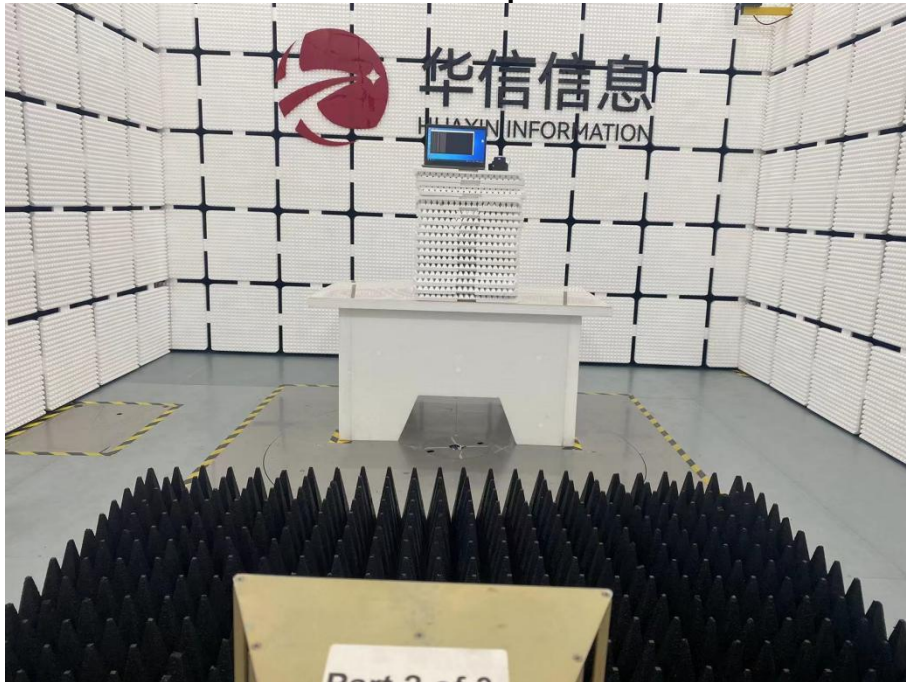
Radiated Emission Test Setup Photo - Above 1GHz
