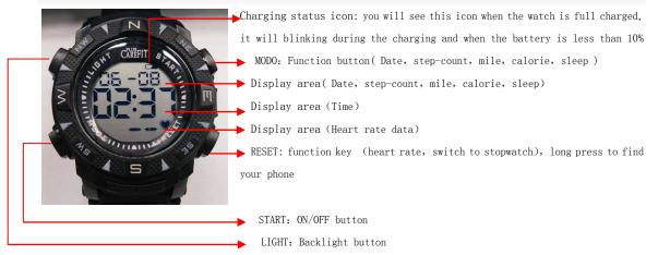
>> Button: MODO Button, LIGHT Button, START Button, RESET Button Button function: short press, long press
