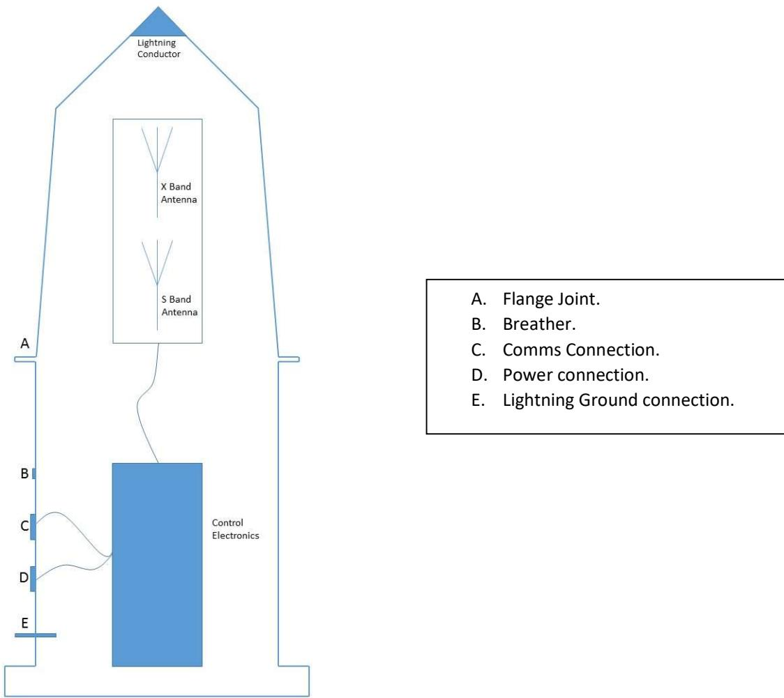
The Transponder comprises one major assembly that contains the S-band and X-band receivers, transmitters and antennas, together with the signal processing and power conditioning sub-systems.
