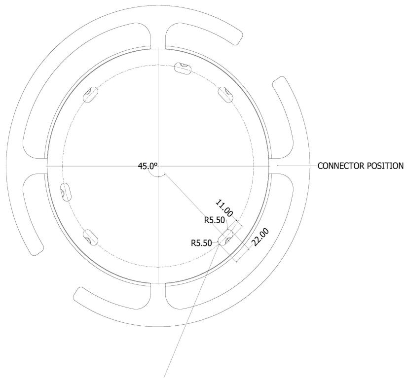
3 THRU' SLOTS EQUALLY SPACED AT 120 DEGREE AND 4 THRU' SLOTS EQUALLY SPACED AT 90 DEGREE ON A 241.3MM DIAMETER
