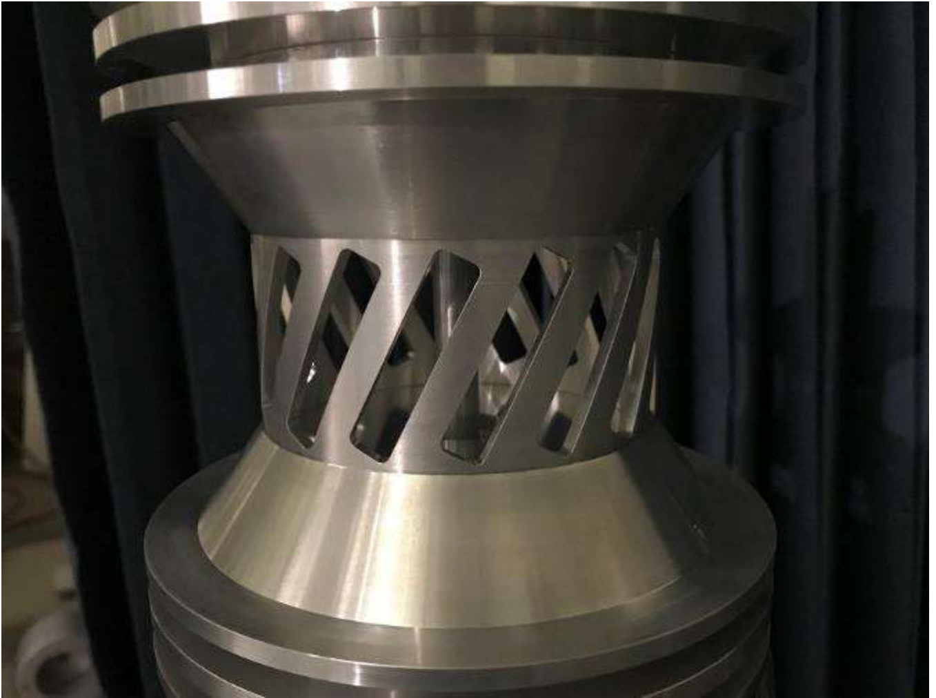
S-Band Antenna, Omnidirectional Slot Array
