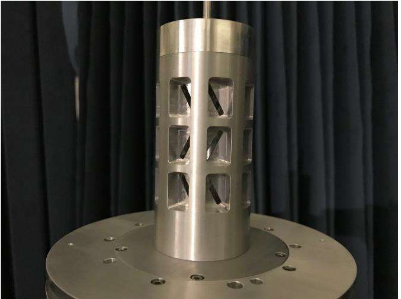
X-Band Antenna, Omnidirectional Slot Array
