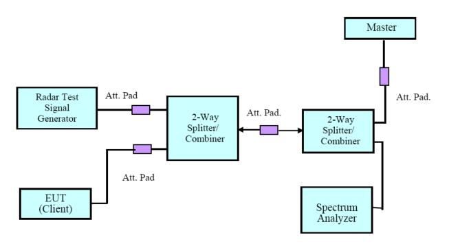
Setup for Client with injection at the Master
