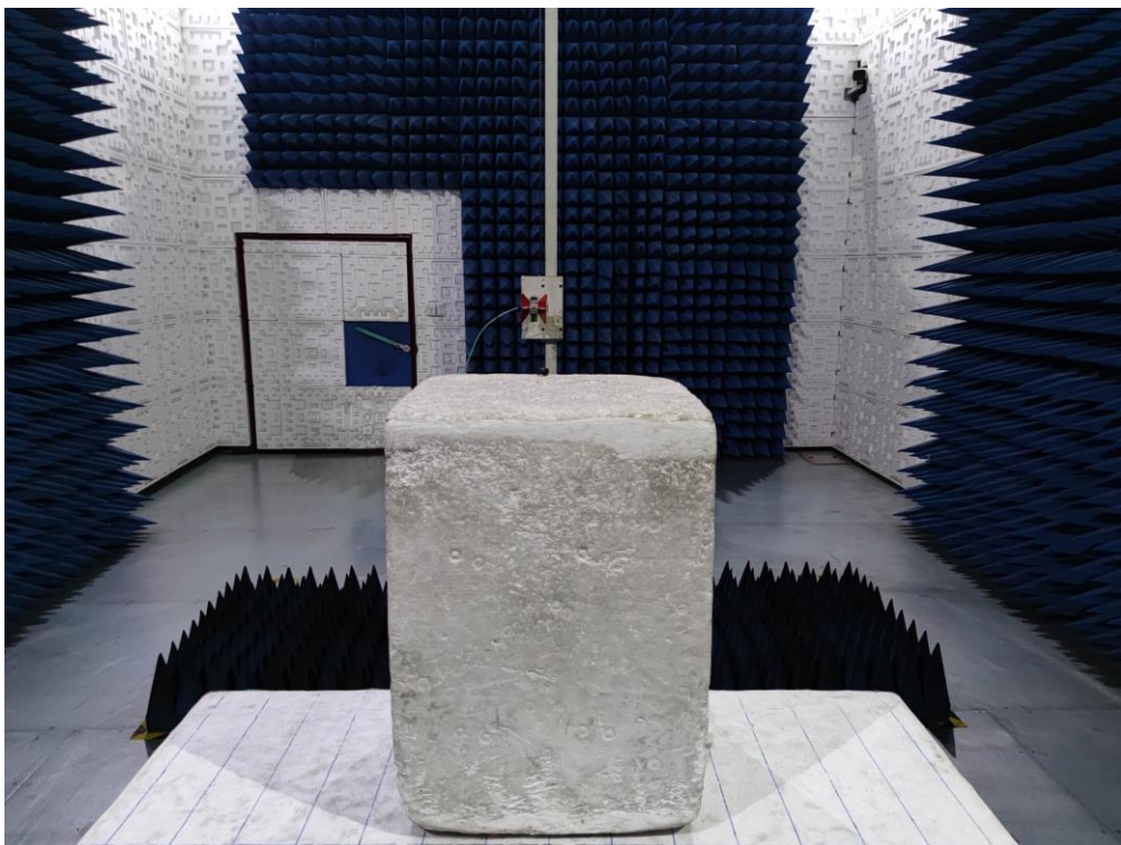
RADIATED EMISSION TEST SETUP ABOVE 1GHZ
