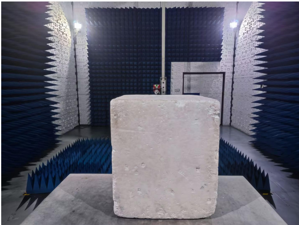
RADIATED EMISSION TEST SETUP ABOVE 1GHz
