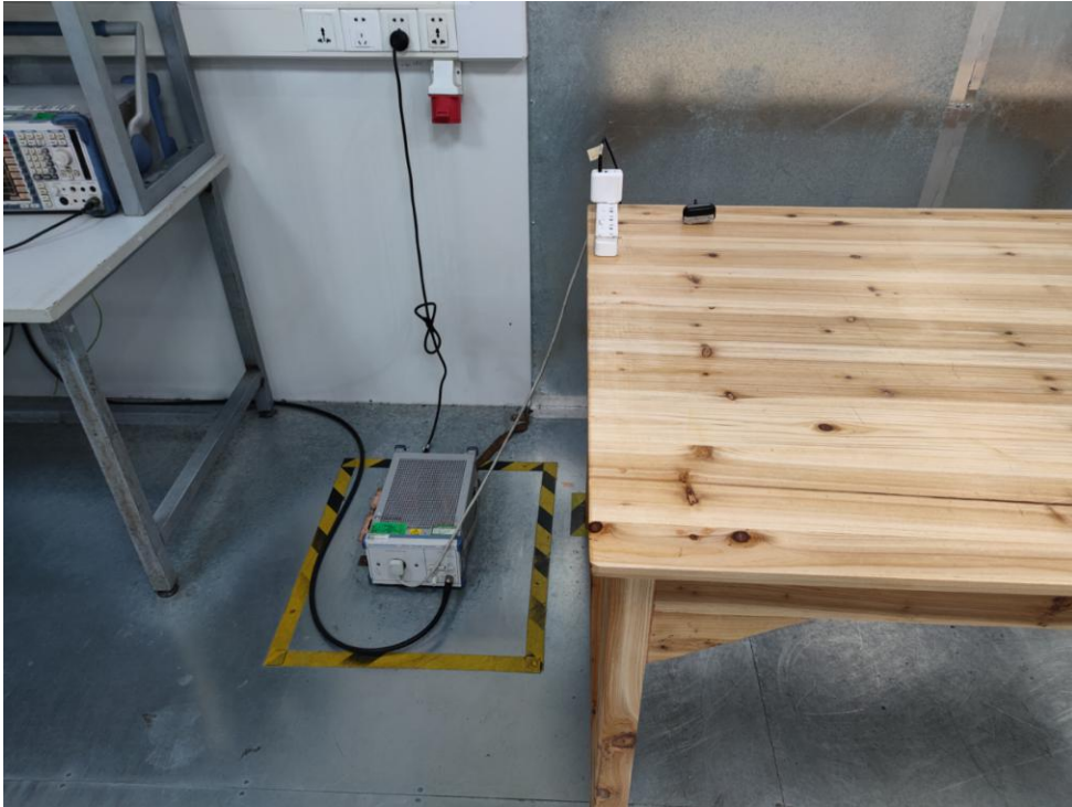
Photo of Conducted Emission Measurement
