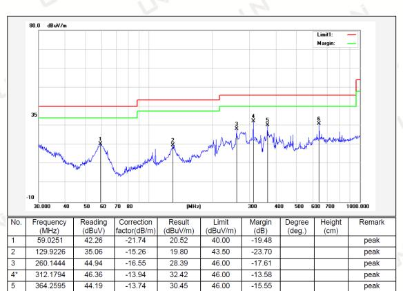
Remark: Absolute Level = Reading Level + Factor, Margin = Absolute Level – Limit Factor = Ant. Factor + Cable Loss – Pre-amplifier
