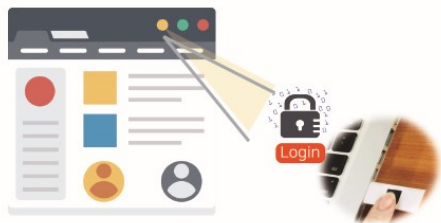
[3] After 1st authentication with ID/PW, log in by executing 2nd authentication with eFA450
