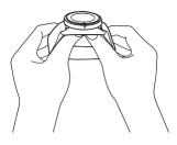
Gently push out the CORE from the bottom of the CORE holder. Please do not try to pull the CORE out from the top of the CORE holder or you might damage the parts.
