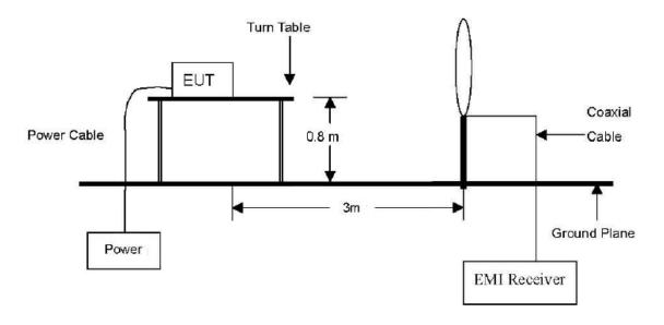
The diagram below shows the test setup that is utilized to make the measurements for emission from 30 MHz to 1 GHz emissions.
