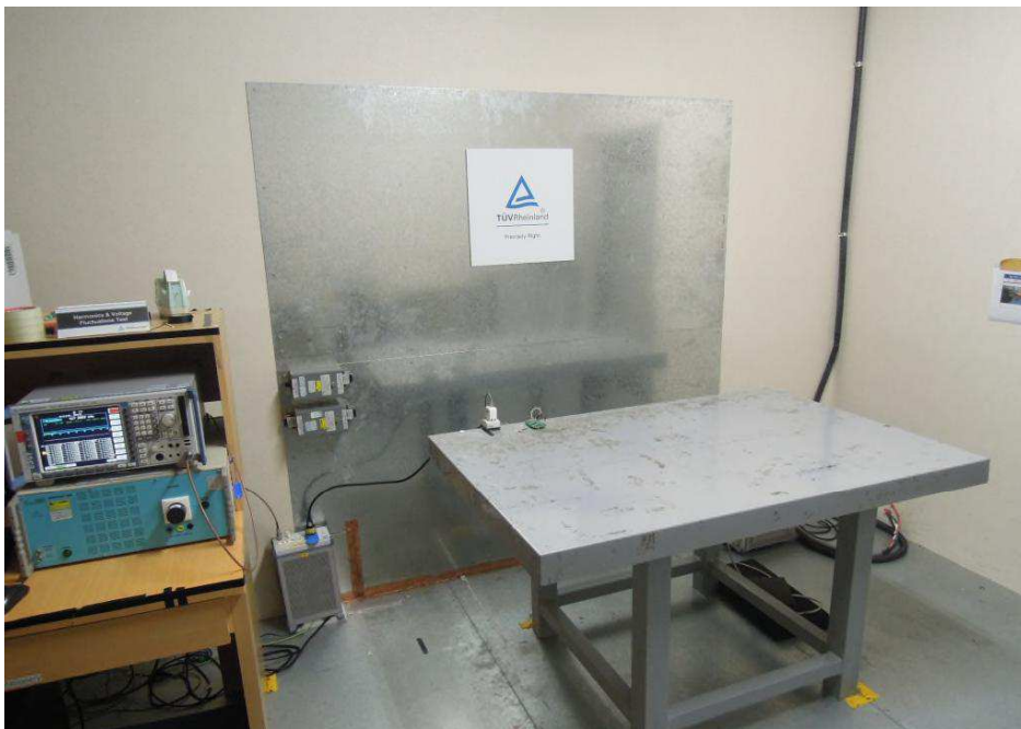
Photograph 9: Set-up for Mains Conducted testing (Back View)
