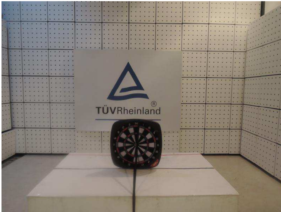
Photograph 1: Set-up for Spurious Emissions (Front View 1)
