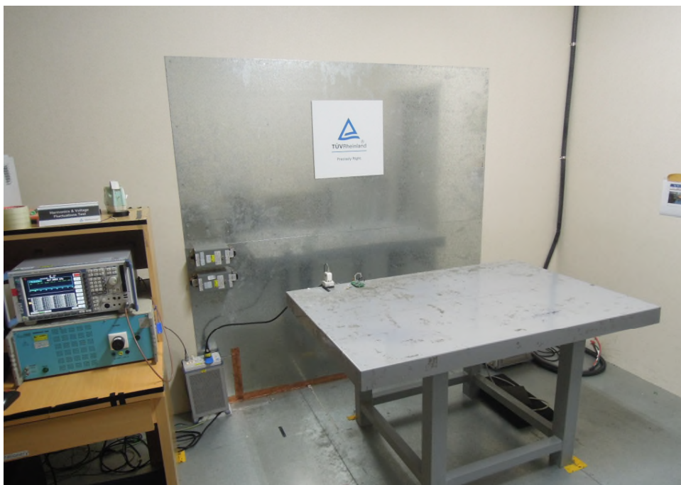
Photograph 9: Set-up for Mains Conducted testing (Back View)
