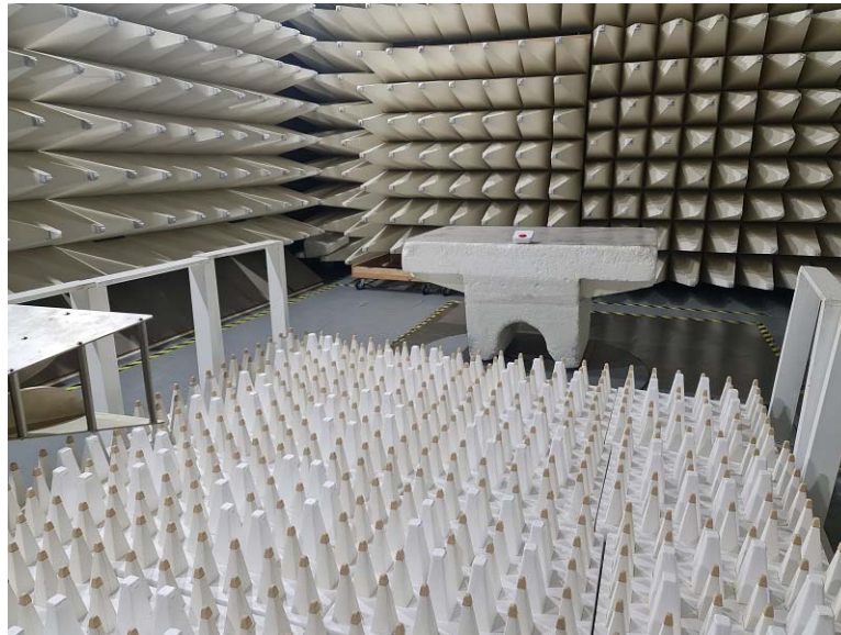
Photograph 8.1.2 Setup for radiated emission measurements above 1 GHz, general view
