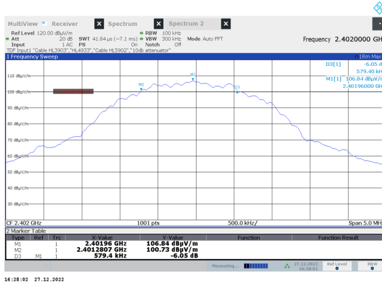
Plot 7.1.1 The 6 dB and 99% bandwidth test result at low frequency at Data Rate = LE_2M_prbs9
