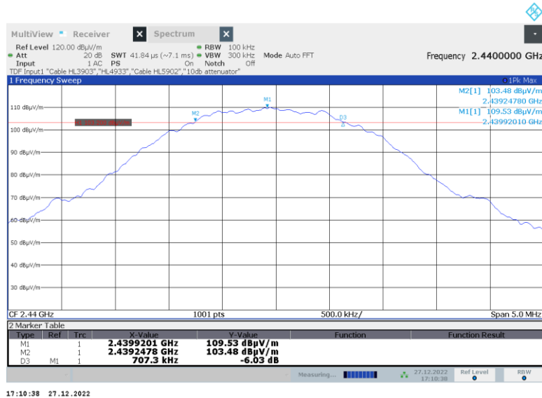
Plot 7.1.2 The 6 dB and 99% bandwidth test result at mid frequency at Data Rate = LE_2M_prbs9
