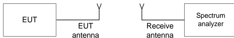
Figure 7.7.1 Band edge emission test setup
