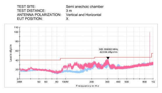
Plot 7.2.6 Radiated emission measurements from 30 to 1000 MHz
