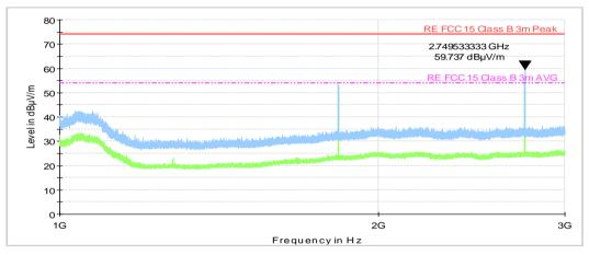
Plot 7.2.8 Radiated emission measurements from 1 to 3 GHz
