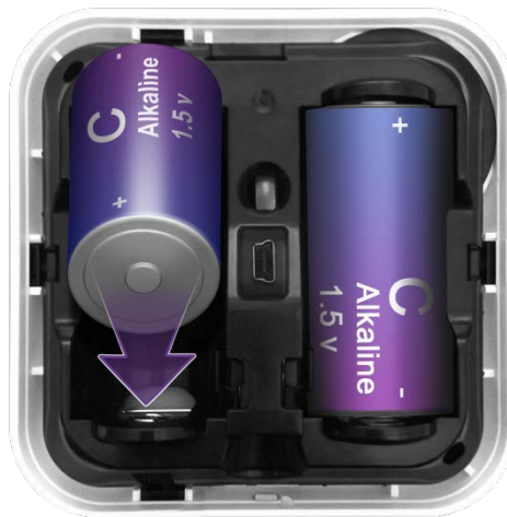
Figure 3: Insert the Batteries
