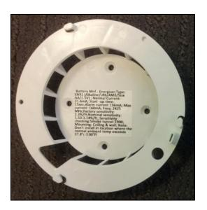
Battery Mnf.: Energizer; Type: EN91 (Alkaline/LR6/AM3/Size AA/1.5V); Steady state current: 49uA; Start -up time: 15sec; Alarm current 105mA; Max current: 130mA; Freq: 916.5 MHz; Factory sensitivity: 2.3%/ft; Nominal sensitivity: 1.53-3.14%/ft; Mounting: Ceiling&wall; Note: Don't install in location where the normal ambient temp exceeds 37.8°c (100°F)
