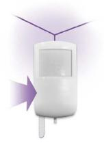
13. Peel off the strip and press the MDsense against the wall.
