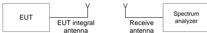
Figure 7.1.1 Setup for transmitter shut down test
