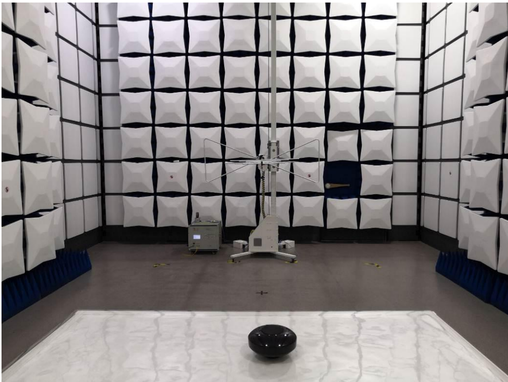
FCC RADIATED EMISSION TEST SETUP
