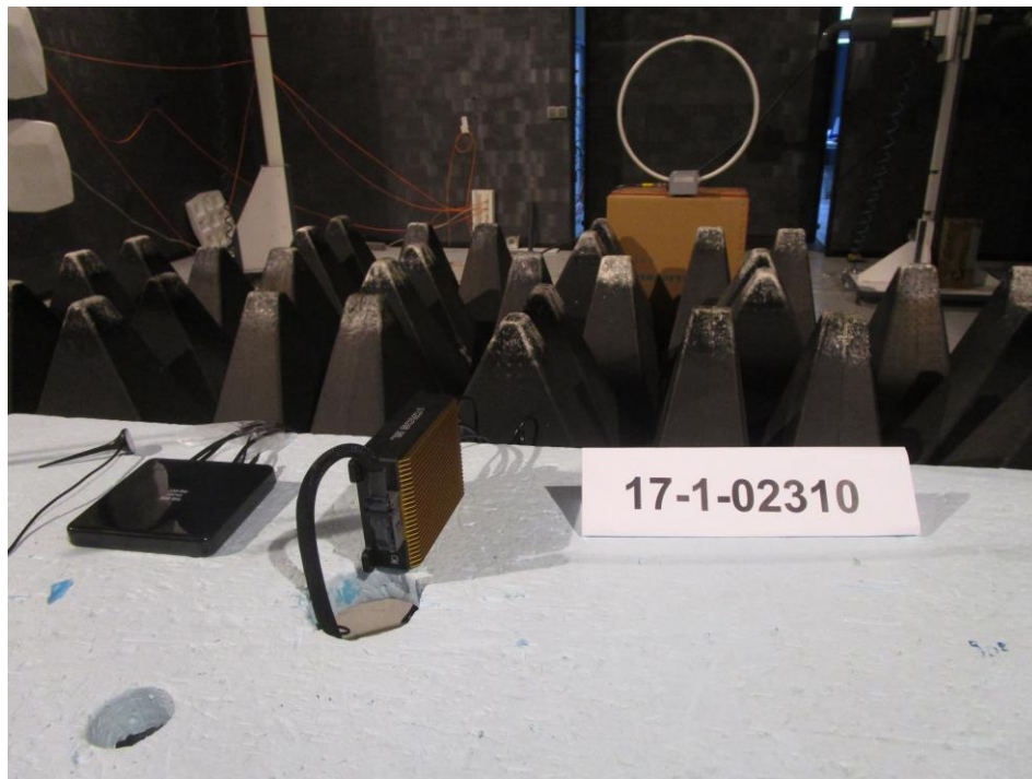
Figure 9: Overall View 9 KHz – 30 MHz EUT Standing
