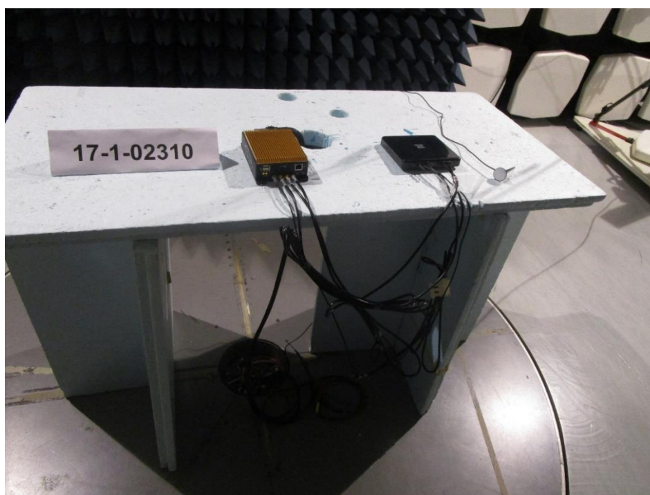
Figure 7: Close View 9 KHz – 30 MHz EUT Laying
