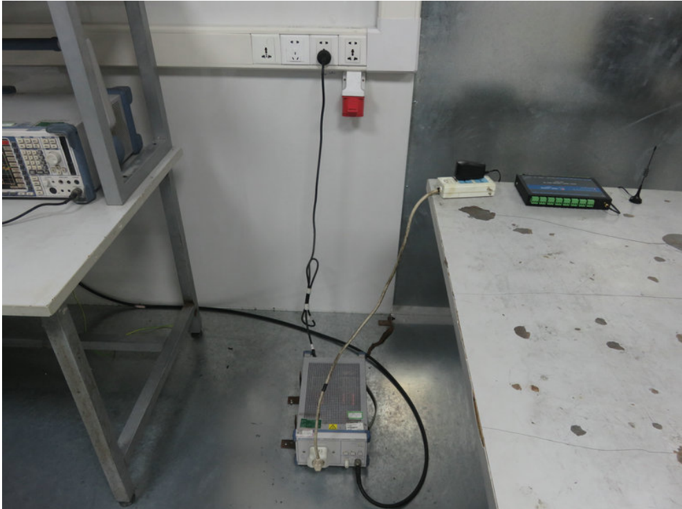
Photo of Conducted Emission Measurement
