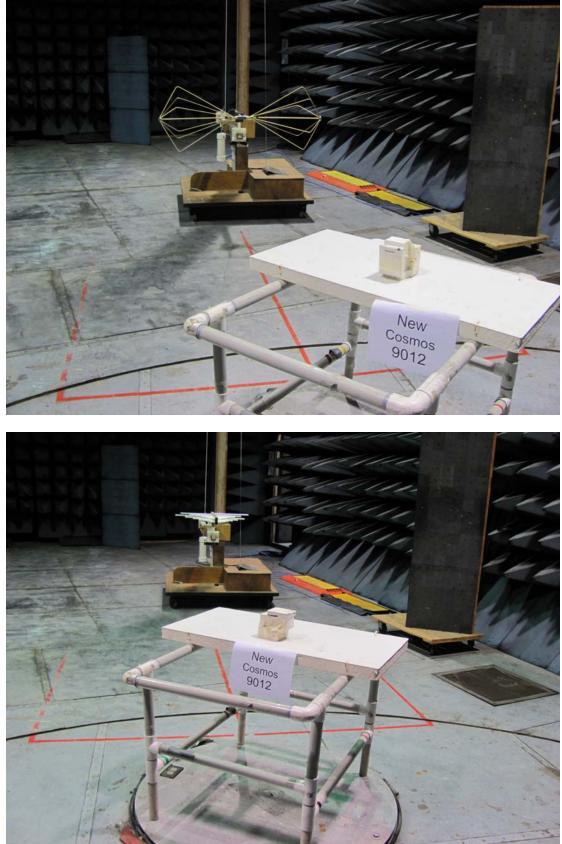
Photographs of Radiated Emissions Test Setup
